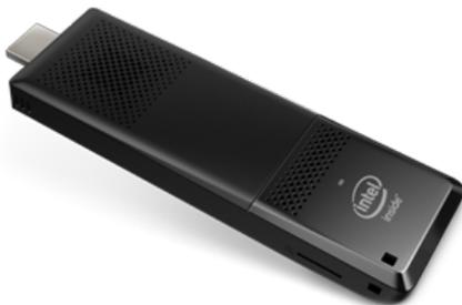
The Intel® Compute Stick is a complete and affordable Windows PC with a quad-core Intel® Atom™ X5 processor, Intel® HD Graphics, integrated Wi-Fi and Bluetooth technologies, 32 GB storage, 2 GB memory, two USB 2.0 port, HDMI port and a Micro SD card reader.
